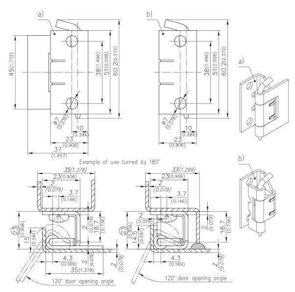
Version Part No. 216-9008 a) Hinge b) Hinge 216-9013
