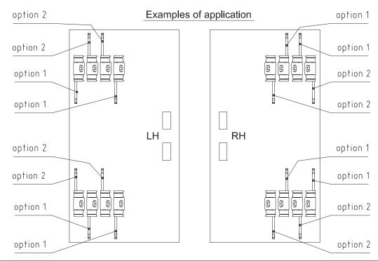
Depending on the shown options, the captive pin is pre-assembled from the top or upside-down. The chart below shows the options for LH and RH doors.
